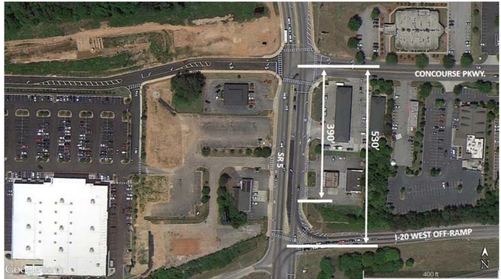
Figure C-3: Intersection spacing, SR 5
