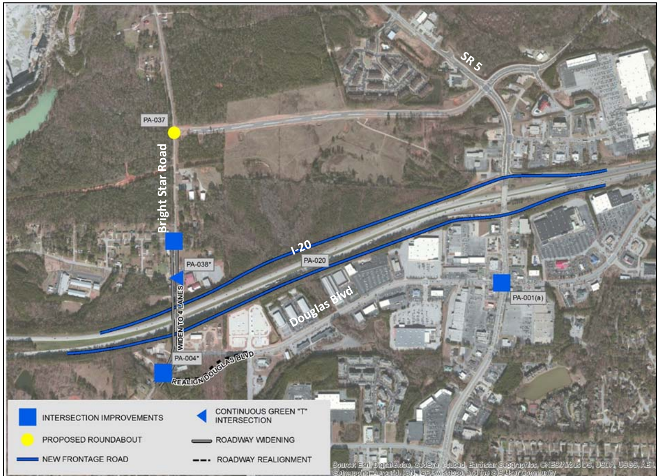
Figure 10: Scenario 4; Construct a split diamond interchange between I-20 @ SR 5 and I-20 @ Bright
